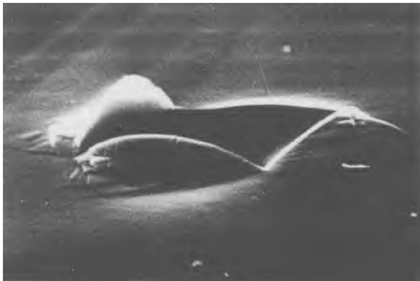
Figure 8-13. Plastic flow of glass under a microhardness indentation. 7,000\times . (After Peter [29]. Reproduced with permission of Elsevier Science Publishers.)
